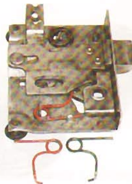
1939-1942 Door Latch Bobby Pin Type Spring The door bolt spring almost never breaks. About ten years ago, a customer requested this spring, and I had to search through about 90 locks to find one that wasn't broken. As a result, I have reproduced this popular item. It will take the sag out of your door handles. In sedans, the left front will fit the right rear, and the right front will fit the left rear. Specify left or right when ordering. $20.00
