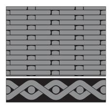
**Plain Dutch Weave:** Woven as a plain weave, but with the warp wires of greater diameter than the weft wires. The weft wires are woven tightly together producing a strong cloth whilst allowing a good flow rate.
