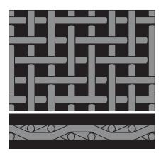
**Twill Weave:** Each weft wire passes alternately above and below every successive pair of warp wires and vice versa. This weave permits a heavier wire diameter to be used than would be possible in a plain weave with similar mesh count.
