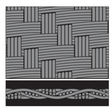
**Multiplex Weave:** A Twill Weave cloth but with multiple wires making up warp and weft. A strong cloth with a relatively high number of openings per unit area, and considerable flexibility. In certain constructions it can produce capillary action.
