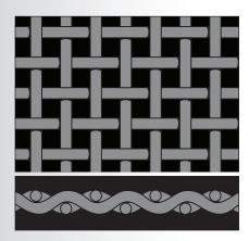
**Plain Weave:** is used for the majority of wirecloth woven by Locker. Each warp wire crosses alternately above and below every weft wire and vice versa. Warp and weft wires are normally of the same diameter. Used for the majority of commercial applications and for filtration where a high flow rate is required.
