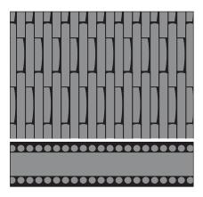
**Reverse Dutch Weave:** Normally woven as a plain weave, but in reverse manner to Plain Dutch Weave the weft wires are of greater diameter than the warp wires, and consequently the warp mesh count is greater than the weft mesh count. This cloth is extremely strong, is easily cleaned and has a high flow rate. Also known as Robusta.
