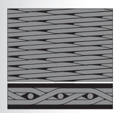
**Dutch Twill Weave:** Similar to Plain Dutch Weave, but effectively has a double layer of weft wires woven in twill pattern. This cloth is "light tight", has a very smooth surface, is strong, but has a restricted flow rate. Also referred to as Micromesh and is used for critical filtration applications often under high pressure.
