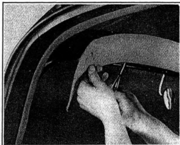
Removing Windshield Header Trim Panel
