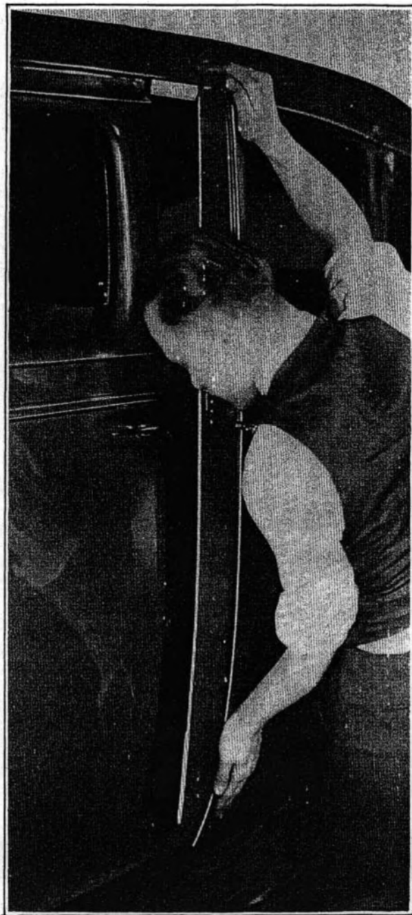
Forcing Door Inward at Bottom to correct misalignment
