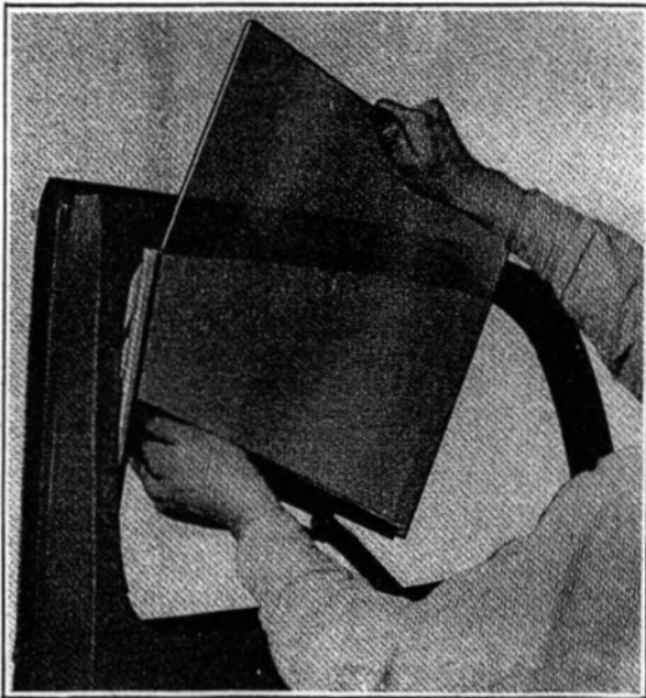
Removing Front Door Glass
