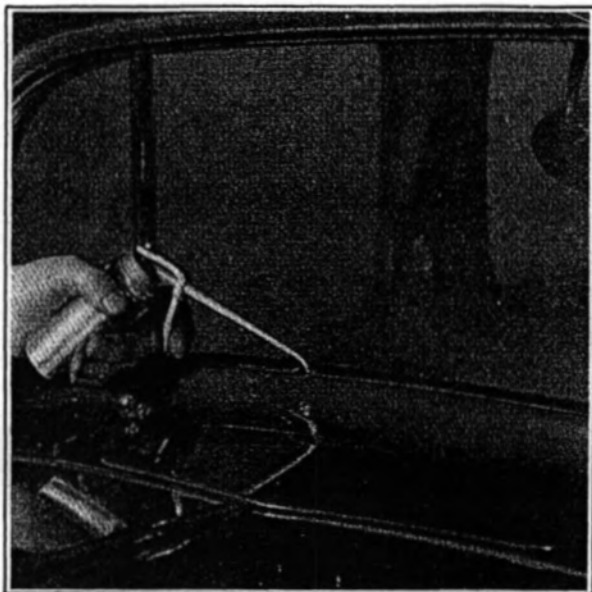
Sealing Windshield Weather Strip to stop leak
