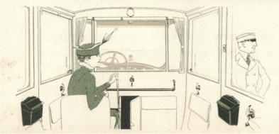
The auxiliary seats, folded, fit neatly into the back of the front seat; in position for use, they are in harmony with the beauty of the interior, ample and comfortable. Between them is a parcel compartment that may be locked. The 3-25 BROUGHAM
