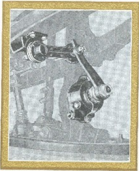
Hydraulic shock absorbers of Packard design and manufacture are standard equipment on all new Packard cars. As indicated, they are built right into the axle and, of course, found in no other car.
