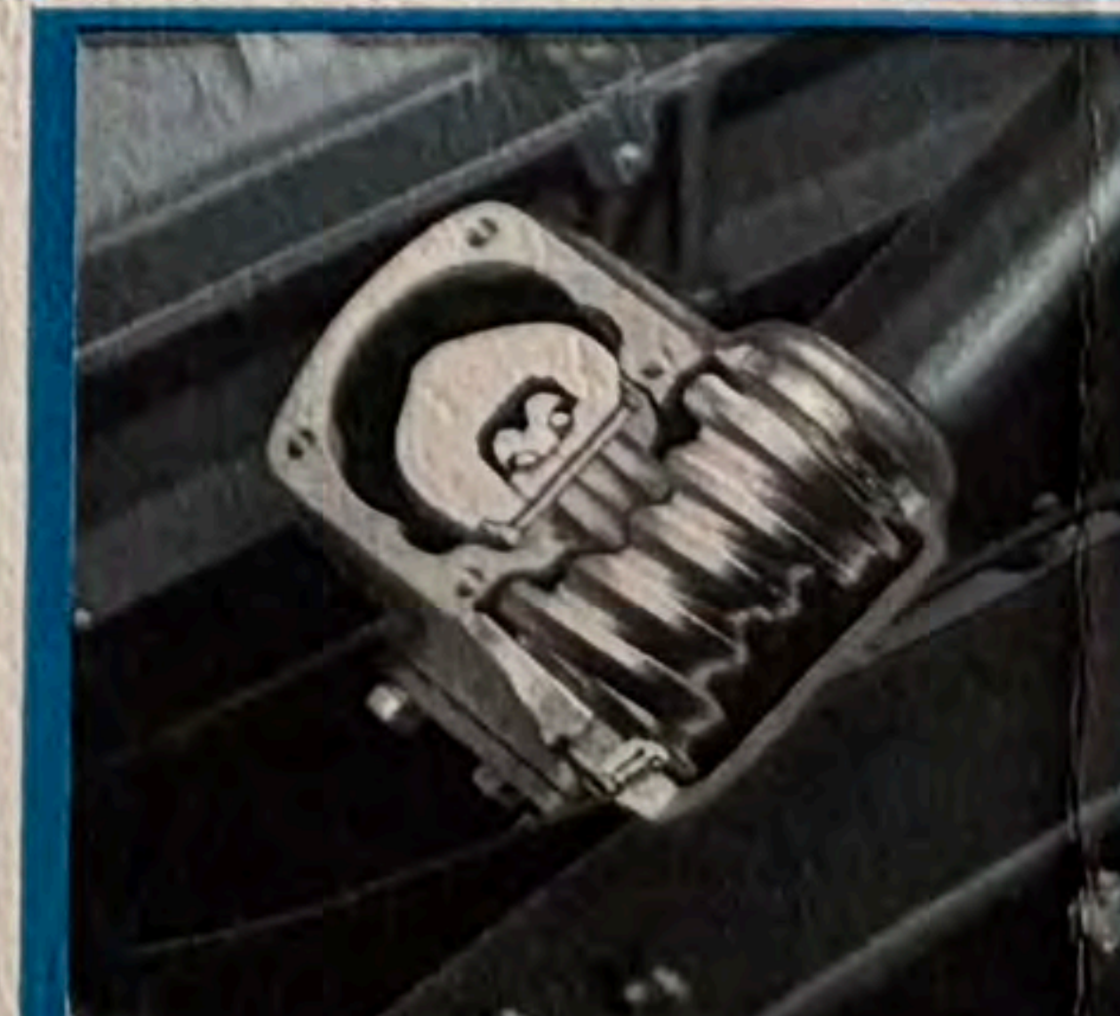
Steering, with its light, responsive touch, is a real joy—thanks to the worm and roller tooth.
