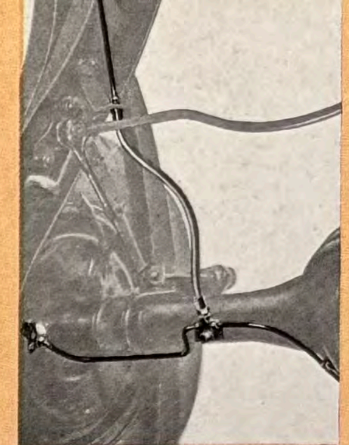
Brake lines protected from flying stones
