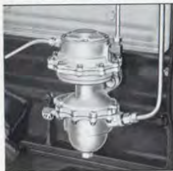
Fuel and Vacuum Pump
