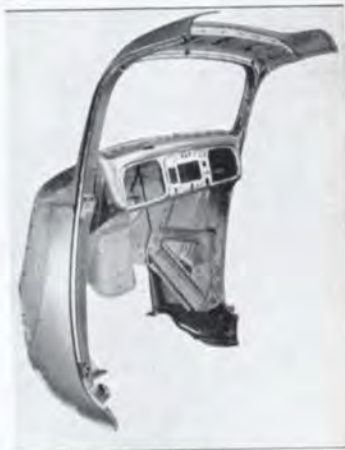
Front Section—All Welded Solid Unit Steel Construction
