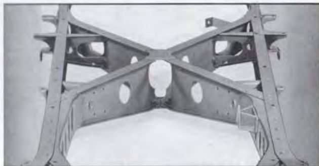
Double-Trussed I-Beam X-Type Frame
