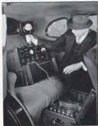
Packard Body Test for Quietness
