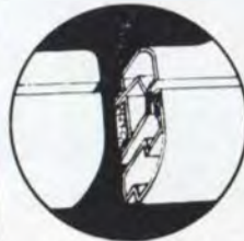
E—Rear Hinge Pillar and Door
