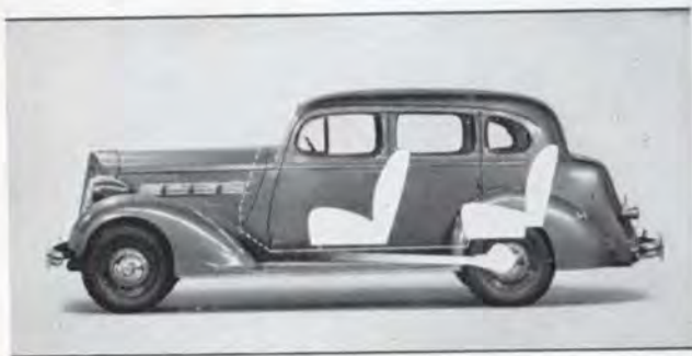
Clear Floors Front and Rear (No Tunnel)
