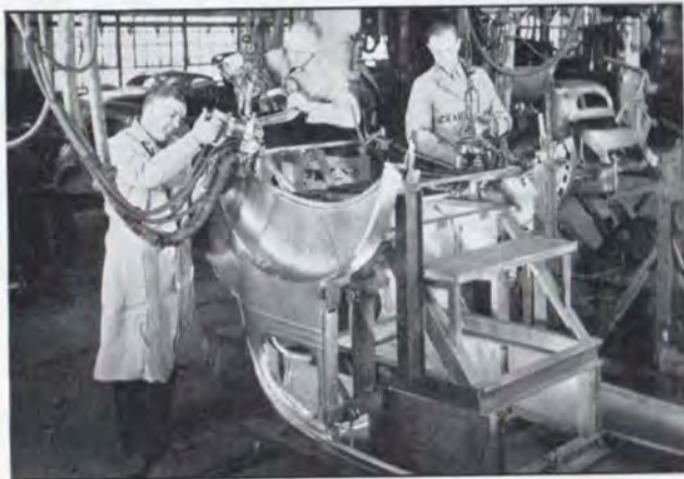
Packard Body—Steel Welding Operation
