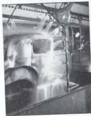
Packard Body Test— Water Testing
