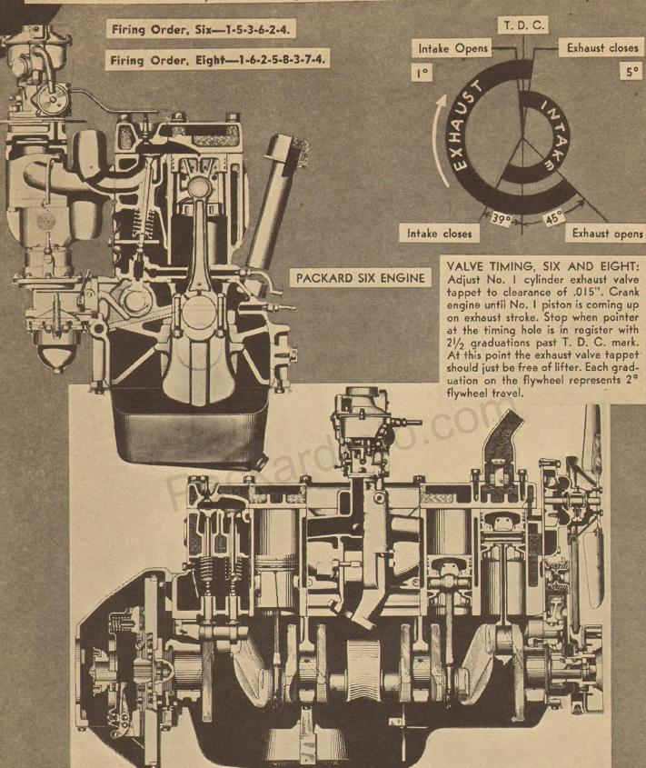
PISTONS: Autothermatic aluminum alloy, with steel strut. Removed from top of engine. Skirt clearance .0015". Piston pin fit in piston, finger push fit at 160° F., weight, on six 191/2 oz., eight 167/8 oz.
