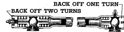
Fig. 47—Adjusting Plug at Steering Gear End of Drag Link (Steering Connecting Rod) Should be Bottomed then Backed Off One Full Turn
