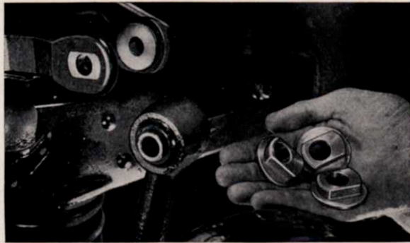
Fig. 48—It is Important to Note Position of Thimbles Because Their Reversal Will Change the Camber Angle
