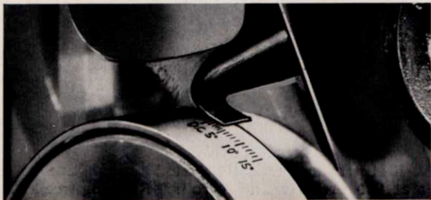
Fig. 17—Each Crankshaft Damper Graduation Equals One Degree
