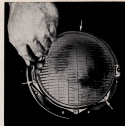
Fig. 24—Three Screws Hold the Retainer Ring in Place
