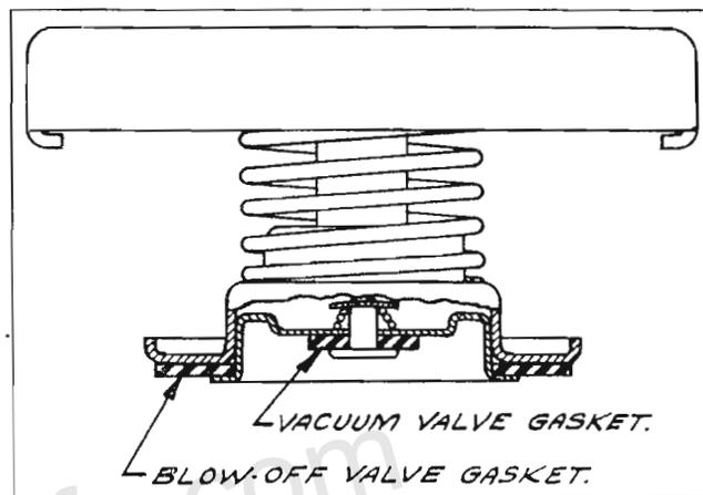
The construction of the cap is shown in the illustration. The large blow-off valve seals the cooling system. It remains closed under normal conditions, raising the boiling point an amount depending on the pressure of the spring. It opens when the temperature rises above the determined point so as to prevent damage from excessive pressure.
