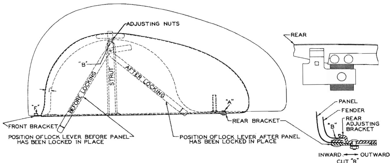
Hook both front and rear adjusting brackets on bottom of panel over lower flange of fender as shown at "F" for front and cut "R" for rear and swing panel up against fender. Front edge of panel to overlap fender about one inch.
