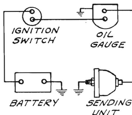
In some cases it may be found that the gauge reading is high instead of low. This is due to the fact that the gauge unit is not properly grounded in the instrument case. You will see in this diagram that part of the current grounds at the gauge and the remainder at the sending unit.
