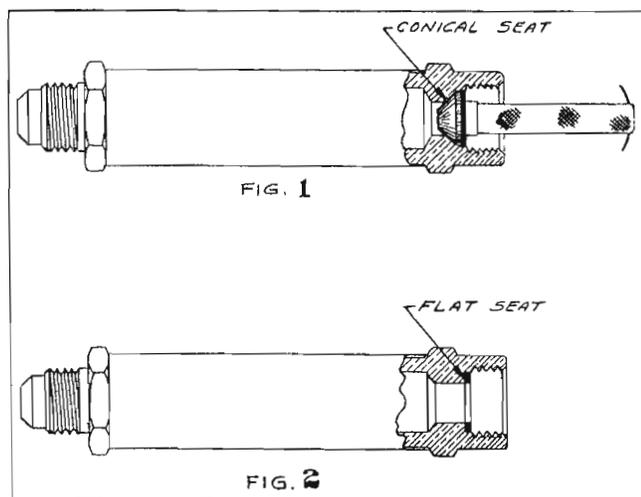
The small screen has been found unnecessary (the large screen inside the filter does the work), but it must be used with the filter having the tapered seat in order to form a tight joint.
