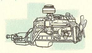
Packard Thunderbolt Power—America's highest compression eight! The *only* engine with a nine main bearing crankshaft. Plus: new service-free simplicity—with up to 25% fewer working parts than in engines of comparable power.
