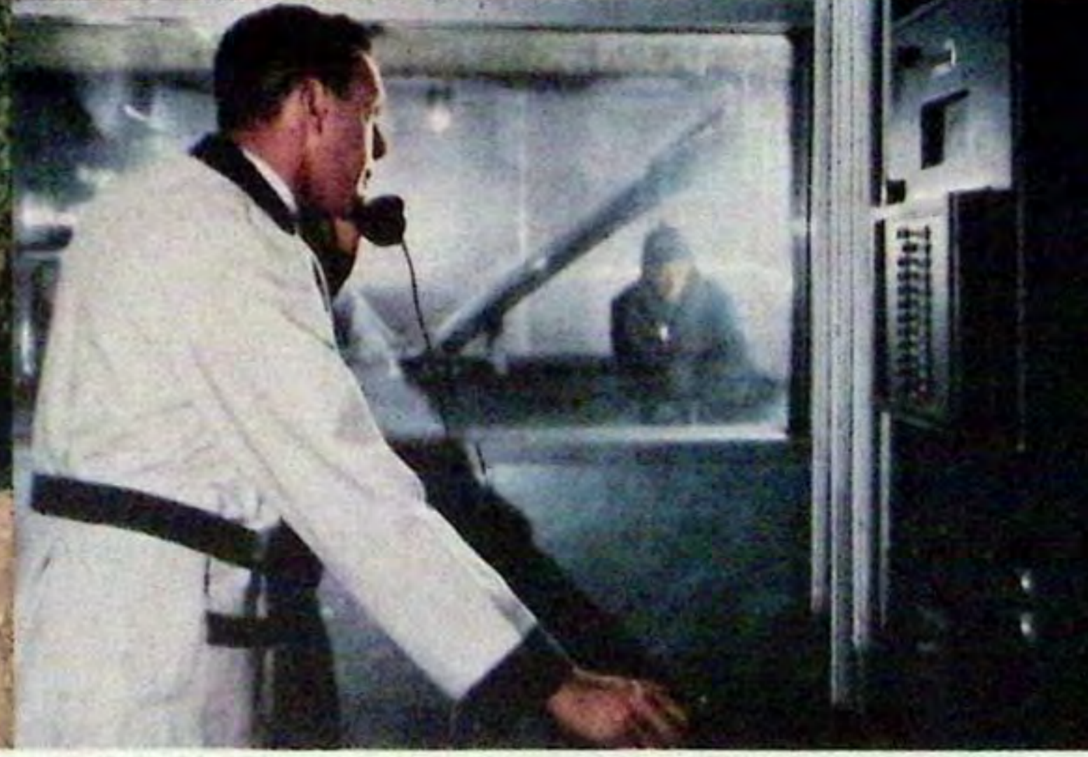
7. Packard engines are tested in the temperature control room, from 40° Fahr. below zero to 135° above, to prove their performance under all conditions.
