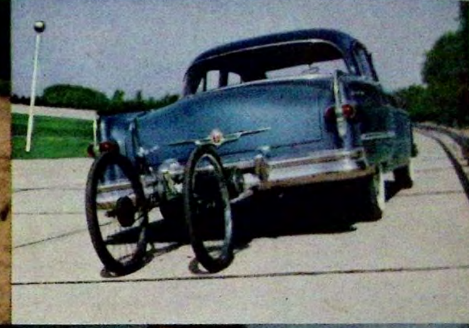
4. Test runs on the world's fastest 2½-mile closed track show the new high-torque Packard 212-horsepower engine provides extra power in the 40 to 70 mile range.
