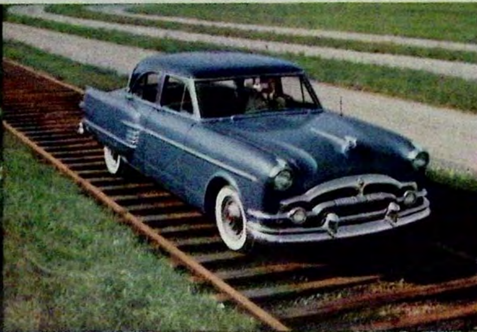
2. Drive over railroad ties proves how Packard minimizes road shock transmitted to the body, steering, suspension and other chassis parts.
