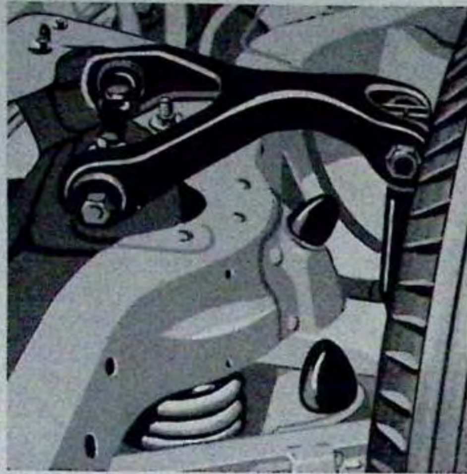
Live rubber bushings are used in Packard's front-end suspension to absorb shocks and jolts at their source—long before they can be passed on to other parts of the car. This is one more example of thorough Packard engineering.
