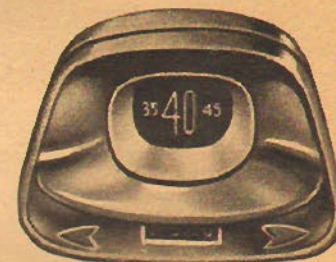
Speedometer dial with magnifying lens shows at a glance the precise driving speed.
