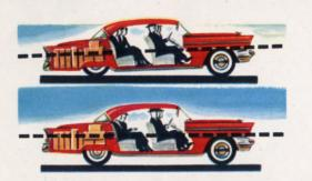
Another Packard exclusive-automatic Load Levelizer maintains the car at normal level when the back end is heavily loaded with rear seat passengers and luggage.
