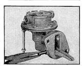
Install cam lever pin.
