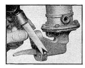
Remove rivet plug. (Use tool T109-43.)
