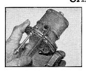
Mark pump body and valve housing to facilitate correct reassembly.
