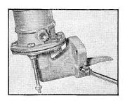
packardinfo.cor Remove cam lever pin plug and washer.
