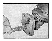
Remove cam lever and spring retainer.
