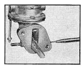
Remove cam lever pin.
