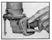
CAUTION-When installing pump on engine be sure slot and stud holes in gasket are aligned with those in face of pump body.
