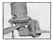
Install cam lever return spring.
