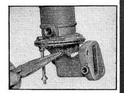
Remove cam lever return spring.
