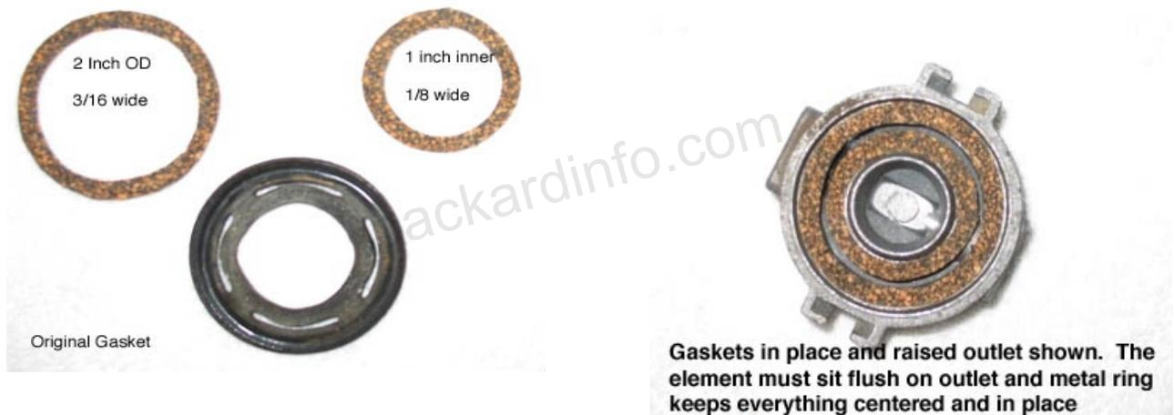
The filter fits in ring, and when glass bowl is installed, it will compress the bottom of paper about 1/8" and hold everything snug.
