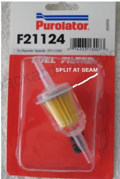
splitting the plastic case, (I used a belt sander and ground off the seam) the filter can be removed. Be careful not to damage the metal ring located in the seam as that is used to provide a seal later on.
