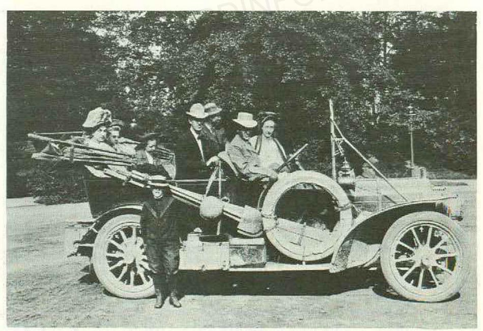
Packard production hits 700 units yearly. Semi-elliptic springs displace platform type. Packard hexagon appears on hubcaps. First of Packard "30's" introduced. Extra reverse gear-shift lever omitted. Headlamps standard equipment. First family to cross continent in an automobile drives a Packard.
