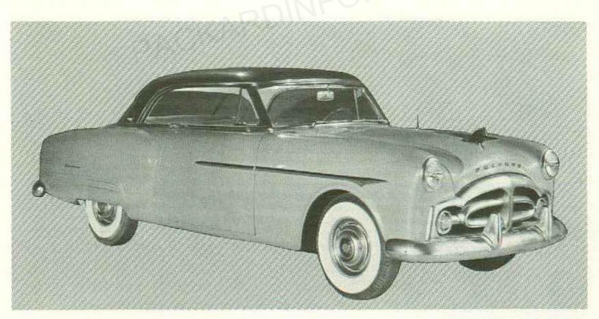
Packard automobiles undergo major styling change with introduction of "contour styling" concept. Fenders raised, hood lowered for greater visibility, safer driving. Wider leaf-type rear springs provide better control. Packard is first to offer low-pedal full-power brakes as optional equipment. Packard power steering introduced.
