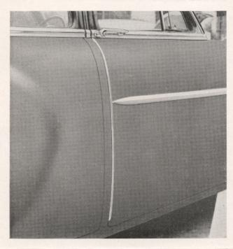
Protection plus beauty has been added to the Packard accessories line for the 26th series car—with the Front Door-Guard. This gleaming stainless steel moulding which is self-retaining prevents the paint from chipping on the opening edge of the front door, thus protecting the beauty of the car.
