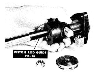
Slip the Piston Rod Guide No. PK-16 over the threaded end of the piston rod and insert the piston rod through seal into adapter housing bore.
