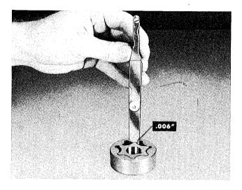
Check the tooth nose clearance of the rotors with a feeler gauge. If the clearance exceeds .006" replace rotors with a new set.
