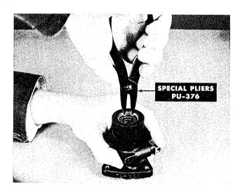
Install the retaining ring with Special Pliers Tool No. PU-376 in the groove near the end of the adapter and balls assembly.
