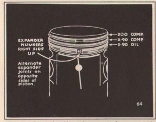
"The numbers in the ring expanders must be right side up. The joints are located alternately on opposite sides of the piston at right angles to the piston pin. The top and bottom rings are located with the joint toward the cam shaft side."
