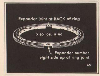
Al: "We install the X-90 oil ring first, and then the X-90 compression with the groove on the lower side, locating the ring joints opposite the expander joints. Then we check to make sure the expander numbers show through the open ring joints with the top of the number toward the top of the piston."
