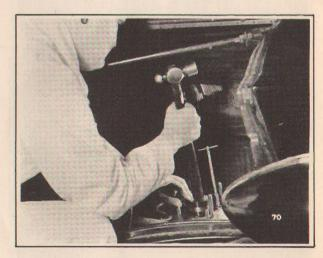
"After washing and oiling the pistons thoroughly, they are inserted in clean cylinders. The rings are compressed carefully, and to avoid the expander springs snapping out of the notches at the ring joints, the ring compression should not be released, once tension has been applied."
