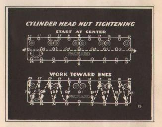
"The cylinder head nuts have to be tightened in the proper order too, Mr. Peck. We start at the center and work out to each end. That way, the head is sort of ironed out, and localized strains and buckling are prevented."
