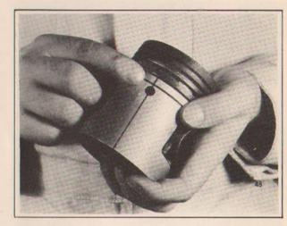
"Now when putting expanders in these narrow invar strut pistons, used on all models except the Packard Six, we must be sure to saw the vertical slot up into the horizontal slot at the top of the skirt just below the lower ring groove."
