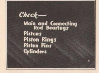
"So we made an oil test of the main and connecting rod bearings - disassembled the pistons from the connecting rods and checked the pistons for scuffs, and gummed and stuck rings - checked the piston pins and bushings for wear - and finally, the cylinder bores for taper. Now, here's what should be done..."
