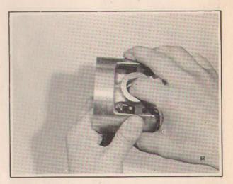
"We locate the stabilizer up and down in the piston so that when it is finally installed, the ends will fit flush around the bosses, and it will not have to be moved. We examine both sides of the piston to see that both the round hole and the elongated hole are visible. We also make sure that the back of the stabilizer fits squarely against the piston skirt."
