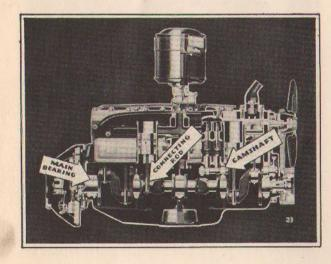
"This test, Mr. Peck, allows us to observe the oil flow from the main, connecting rod, and cam shaft bearings."
