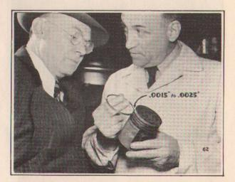
"We check the edge clearance of each ring in its groove. They should have from 1-1/2 to 2-1/2 thousandths clearance. If the ring grooves are worn so as to give more than .007 clearance, the pistons should be renewed. We never re-groove pistons or chamfer ring lands or grooves."
