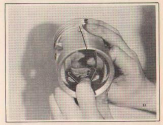
"When installing it, the end of the stabilizer that has the small round hole, is placed against the left invar strut, back of the pin boss. Then the other end is sprung toward the center so that the outside rests against the face of the right pin boss. It is held in position with the finger through the pin hole."
