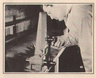
"Connecting rods must be aligned because an out of line rod will cock the piston."
