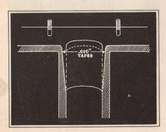
"The next thing we do is to check the cylinder for taper. If they are not more than ten thousandths of an inch tapered, new rings and piston expanders will take care of the job provided the other factors affecting piston ring performance are corrected."
