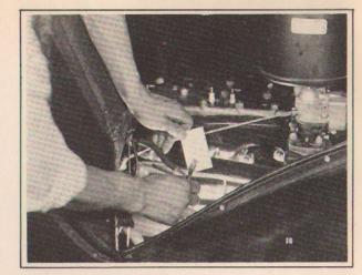
"The vacuum booster pump is a point which must always be checked for oil loss, too."
