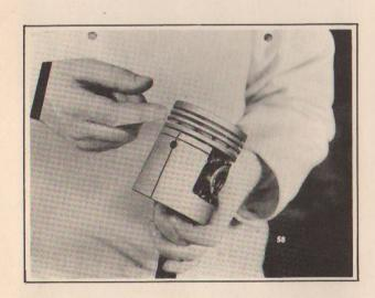
Al: "Before installing the rings, the first thing is to clean all the carbon out of the ring grooves and to clean out the oil drain holes. We must be careful not to scratch or damage the ring lands, and when we use a drill to clean the drain holes, we use a drill 1/32 smaller than the ring groove width, using great care not to touch the ring lands."
