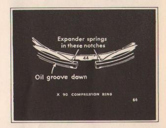
"Each ring is then compressed with the fingers until the ends of the expander springs, on each side of the number, snap into the notches next to the ring joint."
