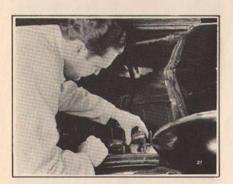
Al: "Because the cuttings from the cylinder will fall down on top of the pistons, then when Pete pushes the pistons out at the top, the rings will carry the cuttings up and out leaving the cylinder bore clean."
