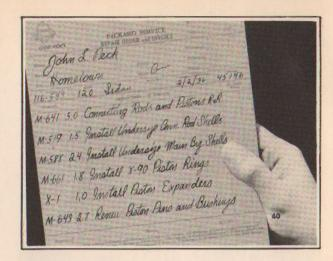
"You need a set of piston expanders to compensate for cylinder and piston wear and piston collapse. The piston expanders will restore the pistons to their original shape and cause the piston to ride square in the cylinder and follow the bore."
