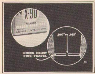
"The basic cylinder size for which the rings are intended is marked on the box. However, we always check the ring gap in the smallest part of the cylinder, below the ring travel. The gap should be 7 to 15 thousandths."
