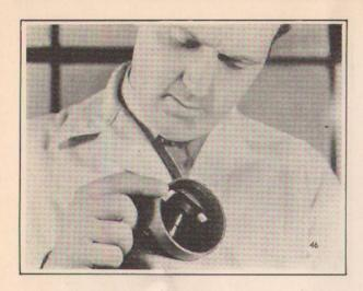
"By the way, Pete - when you install the new expanders and rings, examine the lower edge of the piston to see if it has become beveled or the sharp edge worn off."
