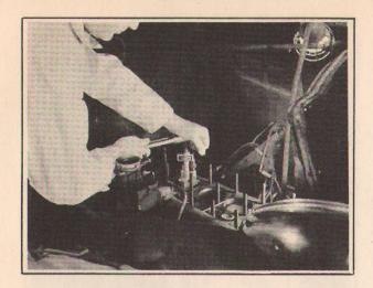
"Before we remove the pistons, we chamfer the cylinder bores with a ridge reamer to take off the shoulder at the top of the cylinder. If this shoulder is not removed when the new rings are installed, the sharp corner of the top ring will hit the shoulder and cause a clicking noise. It might even break the ring. And Pete, be sure that the chamfer doesn't extend too far down the cylinder bore. It shouldn't go into the ring travel more than 1/32 of an inch."
