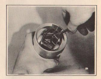
"Then, we make sure that the piston pin will pass thru the holes in the expander. Sometimes these oversize pins bind in the hole, and if they do, we file the expander out with a half round mill file just enough to let the pin pass thru."
