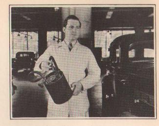
"All set, Pete? ----- Okeh, now connect the oil tester at the manifold connection to the oil pump...."
