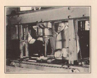
"Then we expand them to a tight fit with the wrist pin burnishing tool. The burnisher does not finish the bearing to size so we ream it to a finger push fit on the pin."
