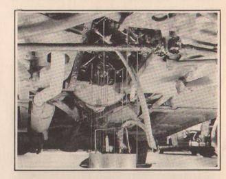
"We put thirty pounds of air pressure on the tester and then turn the engine over with the starter and watch the flow of oil from the main and connecting rod bearings. It should drop steadily from all bearings but should not flow in a stream from any of them. How does it look, Pete?"
