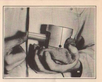
"Then we ream the piston so that it is a finger push fit on the piston pin when the piston is hot - 160 degrees Fahrenheit."
