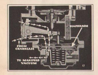
"A small leak in this diaphragm will allow oil spray from the crankcase to be drawn into the engine thru the intake manifold. The loss will be greatest at high speed when the vacuum booster pump is operating, and may be negligible or non-existent at low speeds. The flexing of the diaphragm causes it to wear slightly over a period of time, so we recommend replacing it after £5,000 miles just to be on the safe side.
