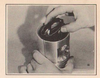
"Next we draw the stabilizer back into the piston far enough to insert a small drift punch through the elongated hole and we hold it there as we pry the stabilizer into position. Then we check it again to make sure the stabilizer fits squarely against the piston skirt."
