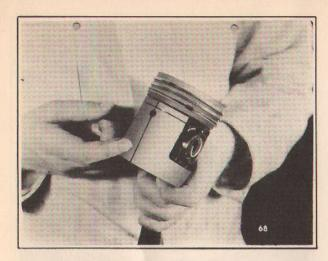
"We next assemble the piston on the connecting rod with the slotted side toward the cam shaft. And when we put in the piston pin lock wires, we make sure that the lip is turned in toward the piston pin to prevent end-wise movement of the pin."
