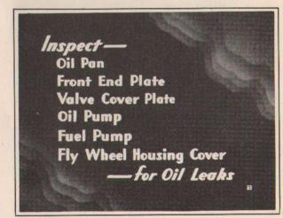
"In the first place, we made a thorough external inspection of the oil pan, front end plate, valve cover plate, oil pump and fuel pump, and for oil drip from the flywheel housing cover."
