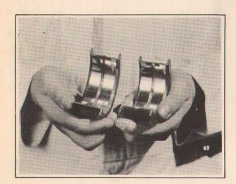
"Before we put the pistons in the cylinders, we install the proper undersize main bearing shells to give a 1-1/2 thousandths clearance on the crankshaft."
