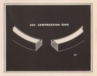
"The number 200 compression ring is placed in the top ring groove with the groove on the inside edge up toward the top of the piston. We never use an expander behind the top rings."
