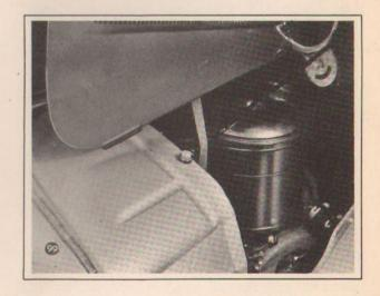
Tom: There's a rubber bumper on the hood to rest on the cowl when it's up and to keep it from rattling when it's down. But looking at it from the service angle . . .
