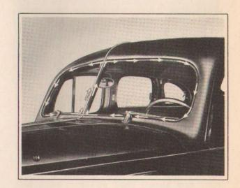
Tom: The same rubber grommet's used for both panes of the windshield. Makes it absolutely water-tight. But it means you have to take out both panes to replace either one. Ah, we're just in time.
