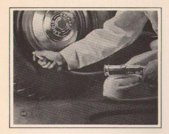
Tom: The tire pressure has to be right. The car is much more sensitive to tire pressure with this new suspension. Always be sure the tires are inflated to the correct pressure for the particular body model you're working on. You'll find a table in the film supplement.
