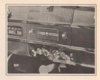
Tom: There's two bosses on the back of the instrument panel to locate the heater and defroster switches in both lines of cars. You just drill through the panel as shown in the instructions, and file out the holes. The switches on the six and eight are the same as they were last year . . with a bulb in the knob, which lights to indicate when they are on. But there's a new arrangement on the senior line.
