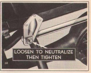
Tom: With a normal load in the front and rear seats, just loosen the bolts and let it find its own position. Then tighten the bolts. 'Sall there is to it.
