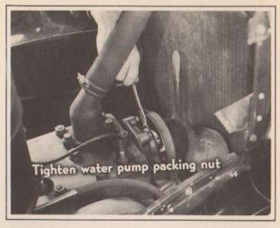
We always tighten the water pump packing nut so she won't leak. That is, if there's enough packing left. If the packing's over half gone, though—we repack it.
