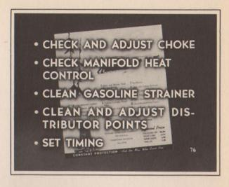
Check and if necessary adjust the automatic choke; check the manifold heat control valve to be sure it is free and the spring connected; clean gasoline strainer; clean and adjust distributor points; and set ignition timing. Say, these are all okay. A lot of these services can be sold again in the spring, can't they?
