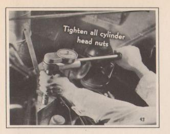
Ed: Well, the first thing we always do is tighten all the cylinder-head nuts down the right amount with the Tension Indicating wrench. And be sure we get 'em all alike. If that doesn't stop the leaks, it's usually because the gasket's no good.
