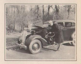
When his fan belt goes, it doesn't give any warning. And it may leave the owner stalled somewhere with the generator, water pump, and fan not working.
