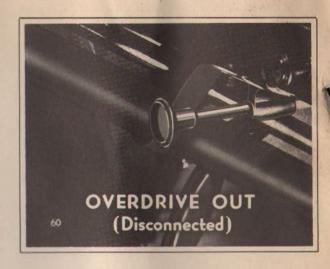
NARRATOR: We're just coming to that. The OVER-DRIVE is automatic in operation, the only manual control being the knob on the instrument board. When the knob is "out" the over-drive unit is locked out and the car operates in the conventional high gear.
