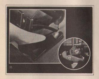
NARRATOR: Be sure to caution your owners about cold weather starting. To engage the choke the accelerator must be depressed to release the fast-idle cam and permit the choke to close. When it's especially cold, you may have to put the foot throttle all the way down to the floor to clear the high step of the cam.
