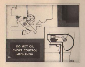
NARRATOR: If it is necessary to clean any of these parts, clean them with alcohol and a clean rag. Do not, under any circumstances, use oil on any parts of the automatic choke control mechanism.
