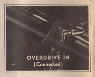
NARRATOR: With the control knob "in," the over-drive is engaged and cuts in automatically at any speed above thirty miles an hour when the accelerator is released momentarily. It will remain in operation through all speeds above twenty miles an hour. At speeds below twenty miles an hour it becomes a free wheeling unit.
