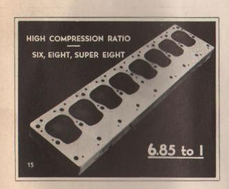
NARRATOR: Cast-iron cylinder heads, for both standard and high compression, are now used on the eight and super-eight as well as on the six. The high compression ratio is six point eighty-five to one. Aluminum cylinder heads are standard for the twelve.
