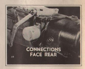
NARRATOR: Pay particular attention to the installation of the solenoid unit if you ever change one. The electrical connections must face the rear of the car. Watch this, because it will wreck the unit to put it in with the connections facing the front.
