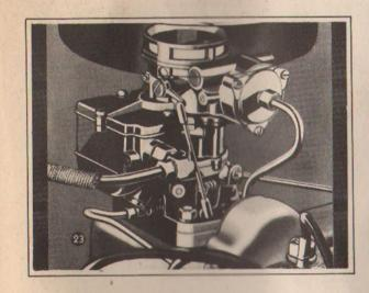
NARRATOR: The eight now has the automatic choke "built-in"--somewhat similar to the six. The thermostat is located on the engine side of the air horn. The heat for the automatic choke is taken from the stove in the exhaust through a tube to a connection, cast in the thermostat cover.
