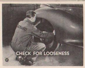
SPEED: And, next, shake the wheels to see if there is any looseness that might throw the adjustment off--loose king pins or bushings, or loose wheel bearings.
