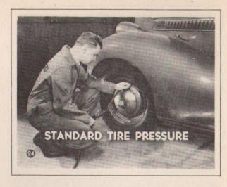
SPEED: First, you bring the tire pressure up to standard on all four wheels so a soft tire won't give you a false reading.
