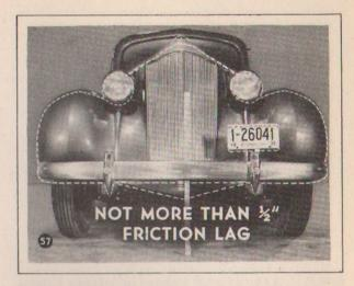
SPEED: Check friction lag by measuring the position of the car at its highest and lowest points. And --
