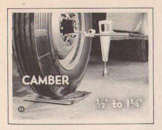
SPEED: Then adjust for camber—putting the high limit on the left hand side, if there's a choice, but keeping the adjustment as near the low limit as possible.
