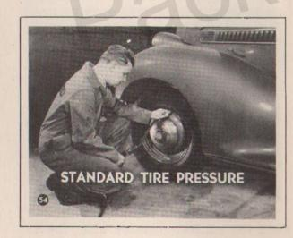
SPEED: Second, inflate all four tires to the correct pressure. And be sure the car's on a level place on the floor.
