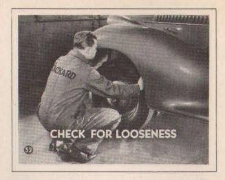
SPEED: First, shake the wheels to see if there's any looseness in king pins, bushings or wheel bearings.
