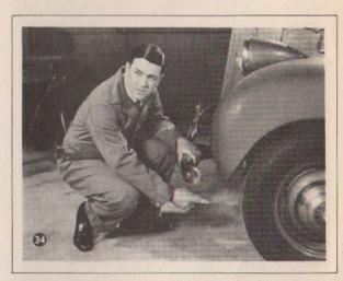
WALT: Changing the position of any of the front suspension parts is apt to put a bind on the bushings that'll put a lot of extra friction in the front suspension and interfere with the free movement of the front end, That'll give you a hard and choppy ride. We call it "friction lag." Get hold of the bumper there, and I'll show you how to check it.
