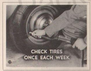
WALT: Tires ought to be checked at least once a week, and the pressure should never be allowed to drop more than three pounds under the recommended pressure. Under-inflation has something to do with almost every kind of tire wear. And keeping the pressures up will reduce the amount of wear.
