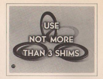
WALT: If the springs have sagged a little, you can install quarter—inch shims between the frame and the spring to raise the riding height up to specifications. Each shim raises the frame about three—eights of an inch. But if it takes any more than three shims, you'll have to replace the springs instead.
