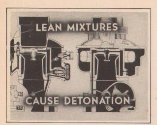
BUG: Now, a car should "ping" slightly on full acceleration if it's set right. Anything that causes too lean a mixture at any speed may cause detonation—a plugged economizer or any plugged passage, or if the main jets are too lean. If the carburetor idle adjustment is set too lean, it will ping up to around twenty—five or thirty miles an hour.
