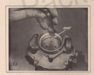
BUG: Clean up the throat and file the choke valve. Make sure there's five thousandth clearance between the long side of the choke valve and the throat of the carburetor.
