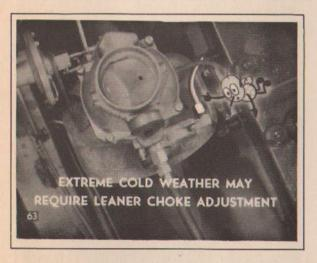
BUG: The reason is that the thermostat is connected by a tube to the hot-spot in the exhaust. In extreme cold weather, the air under the hood does not warm up as quickly as the engine and cools off the air in the tube. So, the thermostat is slow in coming off. If it's extreme cold weather, you may have to lean up the choke adjustment one and one-half to two graduations.
