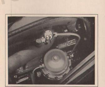
BUG: Here's one that'll fool the best of 'em--a punctured vacuum pump diaphragm. It sure can upset your idle. That's easy to test though. Just disconnect the vacuum booster pump line from the manifold and hold your finger over the manifold connection. If the diaphragm is punctured the engine will smooth out.
