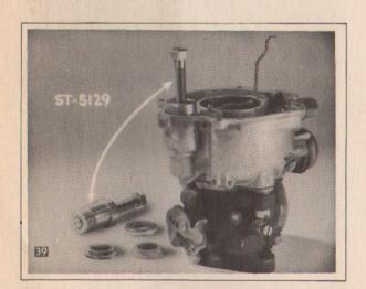
BUG: That's right, Roy, and you should use the special puller to pull the old leather out. Then put in the spring washer, a new leather and tap the metal cap washer in place.
