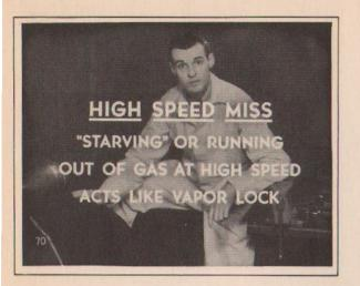
ROY: High speed miss, "starving" or running out of gas at high speed also acts like vapor lock. With the early Chandler-Groves, you might get a high speed miss or cut out at speeds over sixty miles an hour, especially in warm weather. It's due to fuel being drawn from the float bowl faster than it is supplied.
