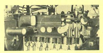
When a motor is rebuilt, or when a water pump is removed for any reason, the tube should be inspected. If it is found to be badly corroded it should be replaced. If the tube fails, the front cylinders and valves—which are nearest the water pump—may be too cool, while the rear of the motor may be too hot.
