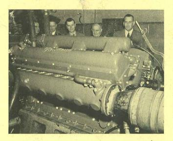
The Marine engine on the dynamometer is inspected by D. C. Cooper—Dayton, R. G. Miller—West Chester and W. L. Greer—Philadelphia. Even the roar verifies the statement that the horsepower of each cylinder is greater than that developed by the 110 car engine.
