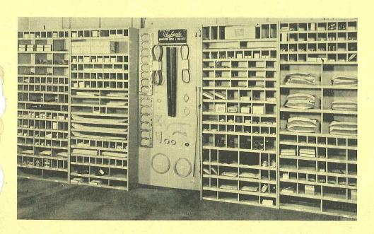
Part Control Plans produce set - ups that look like this—Parts are easy to find, time is saved and obsolescence is reduced to a minimum.
