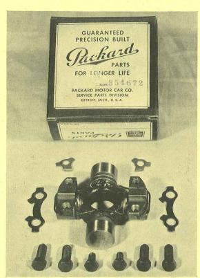
You make no mistake in purchasing Packard Repair Kits. They are Precision Built to factory engineering specifications, assure a good job and save time in both the parts room and in the shop.
