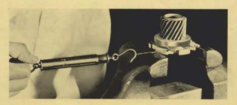
the step of the balk ring. The reading on the scale should be taken while turning the balk ring since the initial effort required to start the ring turning may be considerably higher than the specified torque.
