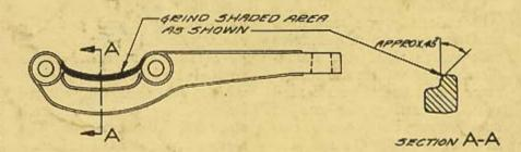
Prior to installing a replacement steering knuckle, a steering knuckle lever, or both, a check should be made to determine whether the lever will interfere with the steering knuckle when the lever is in its normal position.
