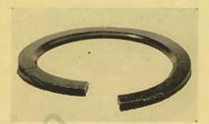
so that the one end is 1/2-inch higher than the other end when the spacer is placed on a flat surface. This will form the spacer to the same approximate shape as that of the recess in the spring seat attached to the bottom of the support arm. The spacer then should be installed in the spring seat with the beveled inner edge of the spacer facing downward and the spacer rotated until the lower end is in line with the edge of the drain hole in the spring seat.
