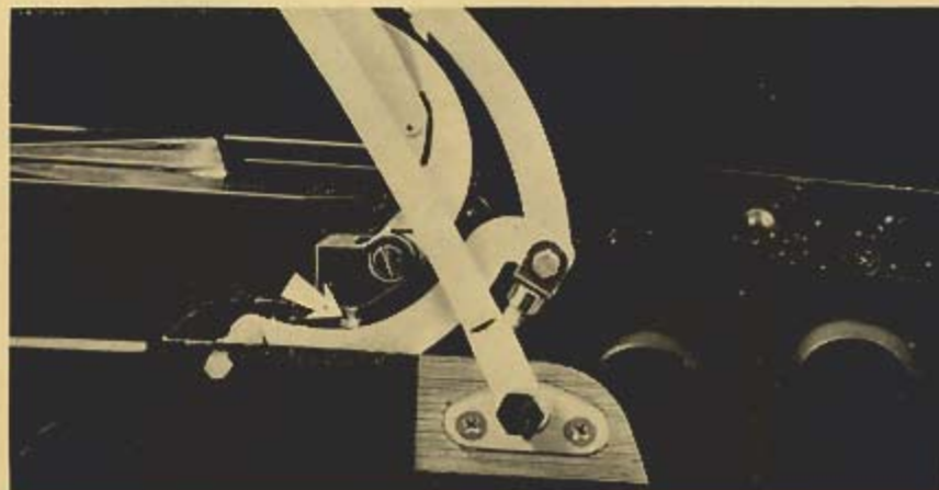
Fig. 24—One of Two Adjusting Screws Controlling Top Forward Movement and Fit at Quarter Window.
