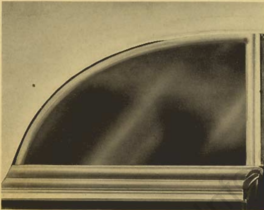
Fig. 25—If Top Gaps as Shown, Turn Adjusting Screws "In". If Too Close, Turn Screws "Out".
