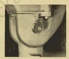
When the engine is started and the exhaust manifold is cold, the thermostatic spring holds the valve in the cold position and permits the hot exhaust gas to circulate around the fuel mixture inlet passages in the center of the intake manifold. This circulation of hot gas causes the intake manifold to heat up rapidly resulting in
