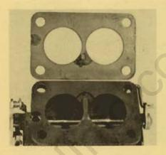
buretor. The accompanying illustration shows a carburetor and a lower gasket which was installed above the insulator block instead of below the block. You will note that a portion of the gasket had swelled and had bulged up into the pocket around the vacuum passage opening, thereby closing the opening.
