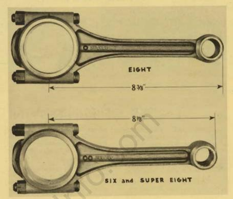
Early production Six and Super Eight engines were equipped with connecting rods having only one "pimple" instead of the two now being used to facilitate identification. These rods may be identified either by the part number 389646 forged in the rod or by the 8½-inch dimension measured from the split line to the top of the piston pin bushing bore.
