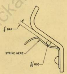
cised not to straighten out the clips or the distance between the clip outer ends, when measured 180 degrees from each other, will be too great to enter into the hub shell cover opening. The clip end must always remain curved away from the wheel.
