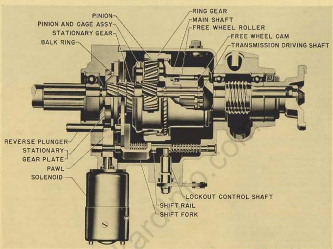
Addition of an overdrive to a standard transmission enables the engine to turn over more slowly and still maintain the same car speed. This reduction in engine speed amounts to about 28%, compared to that required to drive the car at the same car speed in direct drive.
