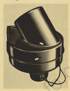
Core leaks, in most cases, can be eliminated by closing the hole with solder. In the event that water has accumulated in the blower housing, the blower assembly should be removed and two ½-in holes drilled at the lowest point of the housing and the inlet duct as shown in the accompanying illustration. This will provide an escape for any water which may find its way into the housing.
