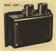
the lever just enough to line it up with the loop in the control wire with the defroster knob in full on position, and the defroster valves wide open. The defroster valves must open to their full open position in order for the controls to fully close the valve door to the plenum chamber.
