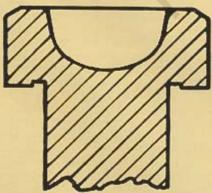
The accompanying illustration shows a cross section through the head of the self-locking type screw. You will note that the center of the head is cup-shaped and that a circular recess extends around the inner portion of the seating face.
