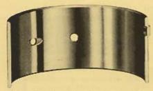
The finish of the bearing surface does not affect the quality of these bearings in any way. Either type bearing will give satisfactory service and bearings of the same size may be interchanged without affecting bearing clearance. The shiny bearing is plated simply to improve its appearance.
