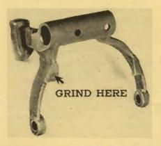
If the overdrive will not engage in low, the electrical system should first be checked. If found to be operating properly, the unit must be disassembled and checked. If the overdrive shifter rail does not move forward far enough to clear the pawl, remove the shifter assembly and grind approximately .020 inch from the end of the shifter rail.
