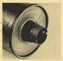
If this trouble should be experienced on a muffler replacement job, it may be easily corrected by "dinging in" the shoulder interference area with a ball-peen hammer.
