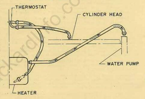
Occasionally a "metallic flutter" may be heard behind the instrument panel in the vicinity of the heater control system. This noise will invariably occur at a given combination of engine speed and heat control setting, and normally can be caused only by an improper hook-up of the heater hose.
