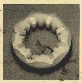
If the speedometer driving gear is installed with the grooves toward the front, the spray of oil will be directed to the breather causing a severe oil leak.
