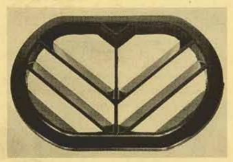
By using a hack saw blade, the two upper grille blades can be cut off as shown in the illustration without removing the grille from the dash panel.
