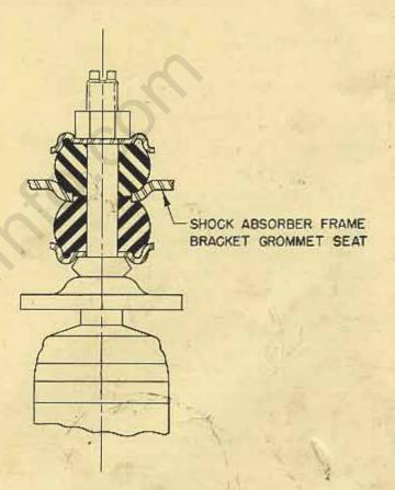
Attach the upper end of the shock absorber to the frame with the retainers, grommets and retaining nut.
