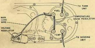
Starting with Engine Numbers L-202588, L-301595, L-401245, L-600503, the regulator was discontinued and a new re-calibrated sending unit is used. The electrical wiring hook-up used with the temperature gauge regulator is shown in the illustration. The dotted lines indicate the wiring hook-up used without the regulator.
