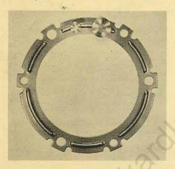
In some instances a planetary assembly may be found without balancing weights, but will have a star stamped on the outside of the planetary cage. The star indicates that the planetary assembly is in balance and does not require any weights.
