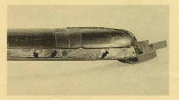
source may be traced to an opening at the forward lower edge of the header. "See arrows on the illustration." Water entering the header will flow back through the ends of the header and into the side rails.
