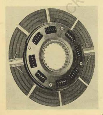
If direct drive clutch slippage is encountered on early production units and the converter "in" and direct drive clutch pressures are within specifications, it is suggested that the direct drive clutch plate be removed and reworked as follows:
