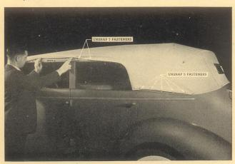
Operation 2. Unsnap all glove fasteners along roof side rail and rear quarter above rear wheel (12 fasteners on each side). Failure to do this operation before lowering the top will cause fasteners to pull through the top material.
