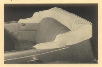
NOTE—If, when raising, the top fails to register on the front dowel pins, loosen knurled thumb screws at the top of rear pillar which will relieve the tension. Tighten wing nuts and all thumb screws using a wrench to pull firmly into place.
