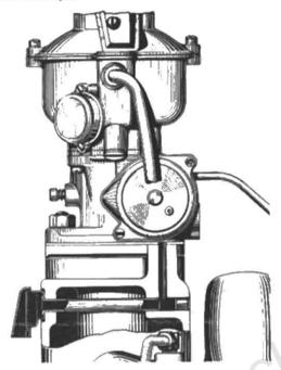
When moisture and rust are found in the automatic choke chamber, examine the heat hole in the carburetor body. Moisture or carbon deposits on the walls will indicate an exhaust leak and the tube must be made tight in the manifold. In some localities, due to conditions of temperature and humidity, condensation forms in the automatic choke chamber even though there is no exhaust leak.
