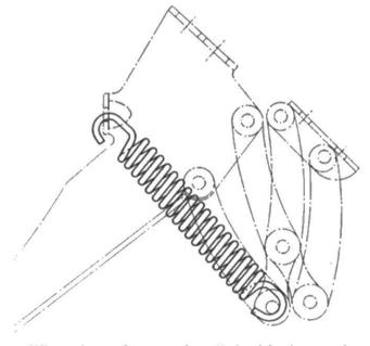
When the springs are installed with the opening facing down, as illustrated, the contact is kept in close to the shank of the eye, the load is much reduced and no trouble will be experienced.
