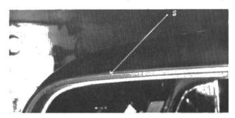
To seal a leak at "S" it is not necessary to remove the section. Seal the opening with a good top sealer all along both sides and a permanent cure will be effected.
