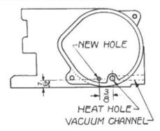
Drill a No. 60 drill size hole 35" to the left of the heat hole and 37" up from the flange. Drill through from the automatic choke chamber to the vacuum channel. This will permit moisture and condensation to be drawn off, and thus prevent rusting.
