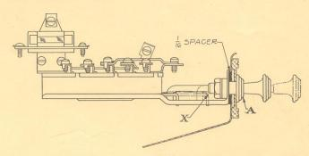
When the switch button is pulled out all the way an interference may develop at the point marked "X". This interference is between the rear end of the flat stamping and the forward end of the boss which supports the shaft operating the stamping. When the interference occurs it is usually because the nut "A" on the instrument board has been pulled up so tightly that the switch body is pulled back beyond its proper
