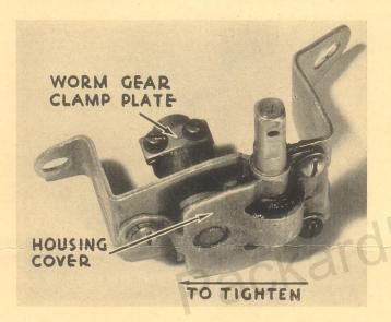
The regulator housing cover which positions the worm in relation to the gear, is attached with three screws the holes for which are slotted to allow for adjustment. Moving the cover toward the single screw moves the worm toward the gear, decreasing the back-lash.
