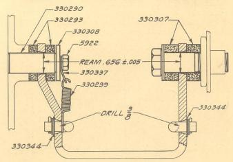
The illustration shows a recent production change in the clutch shifter relay lever.
