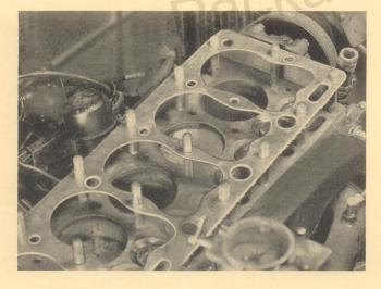
Failure to clean rust and corrosion from the cylinder head studs is often the cause of blown-out and leaking cylinder head gaskets.
