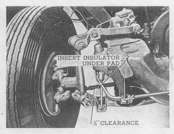
Before finally tightening the bolts check to see that there is at least ½ inch clearance between the outer side of the bracket and the wheel support arm. Grind off the bracket if necessary to provide clearances.
