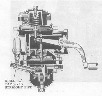
fuel pump is removed from the engine it is only necessary to drill out the cored recess in the discharge side,  $\frac{11}{32}$  inch, tap  $\frac{1}{8}$  x 27—straight pipe thread, and install air dome.
