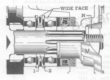
Only the new type parts are being carried in service stock. The new spacer and spring assembly will be shipped on orders for the old type collapsible spacer 338476. Distributer and dealer stocks of the old type spacer should be scrapped.
