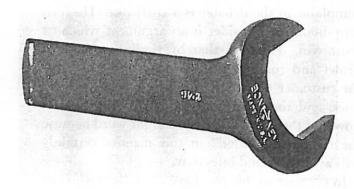
Time will be saved if you use this special short wrench to change the Econo-Drive Governor at the frame X member. It is a very difficult operation without the proper wrench, ST-5197, which has a  $1\frac{7}{16}$ " opening. The wrench is \$1.30 list.
