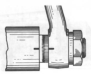
placed in the straight-ahead position. If the steering linkage is correctly adjusted, the steering connecting rod will just reach from the steering crank to the steering lever.
