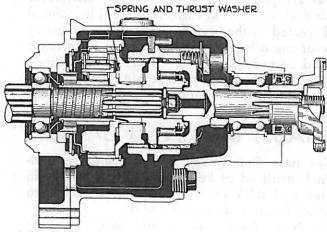
Third: Install spring-loaded Econo-Drive clutch thrust washer. This washer is used to replace the solid bronze thrust washer between the planetary pinion cage and the ring gear hub.
