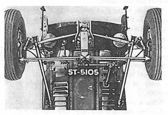
and they must be relocated and the toe-in checked and reset. Install the Steering Crank Aligning Gauge ST 5105 in the frame cross channel under the steering crank. The point of the gauge indicates the center line of the car. Adjust the cross tube until the distance from the center of the gauge to the brake backing plate is the same on each side.
