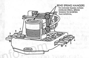
When the upper points are closed and then released, the lower points should open a split second later. During the split second between the opening of the upper and lower points, the ignition is grounded to permit withdrawal of the pawl when the solenoid is de-energized by opening of the lower set of relay points.
