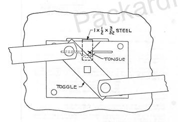
Some service men have installed a coil spring to hold the toggle in the out position. This is an unsatisfactory correction in that the latches are held out when the trunk lid is open and the handle must be turned to close it. With this arrangement should the lid drop shut or the operator fail to turn the handle when closing the lid the latches strike against the body panels damaging the paint.
